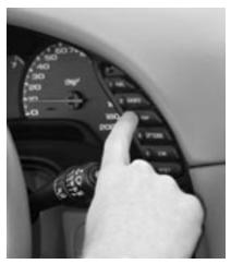
Features that are accessible through the DIC are remote power windows, initiation of Retained Accessory Power, Passenger Power-Lock Assist, and a High-Speed Report. The high-speed report shows the highest speed experienced with the vehicle. It can be reset at any time so you can keep tabs on your Corvette if it's in the hands of a valet or a high-school senior on prom night.
