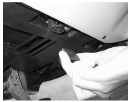
Your Corvette has an ALDL connector under the dash located centrally on the driver side. This is where GM technicians plug in their diagnostic equipment if such services are needed. Before servicing, you can simply pull out the Window Valet to prevent it from being misplaced. Then, when you get the car back, you can simply plug the Window Valet back into the connector. The Window Valet's settings are retained so additional reprogramming is not necessary.
