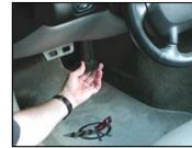
The Window Valet™ for C6/XLR plugs into the diagnostics port underneath the steering column, just passed the edge of the dash trim. There's no configuration required. Just plug it in! The Window Valet™ for C6/XLR does not reprogram any of the car's computers. So to reverse the install, just unplug the unit, and the car will immediately revert back to stock.
