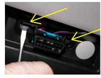
get just a little slack from the wiring harness feeding the connector.
