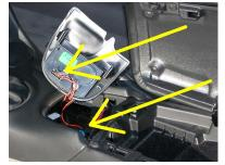
grip by prying upward on the edges that are towards the console storage area. Then remove the cable connector to free the console panel and set the panel safely aside. Also disconnect the storage area's accessory power connector. Note that each connector has a locking tab.
