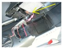
Lift the whole assembly up and reach underneath and inside the fuel switch area and disconnect the connector (this connector also has a locking tab) from the switch housing. Lift the entire console out and set it aside. A second person may make an easier job of disconnecting the fuel release switch cable.
