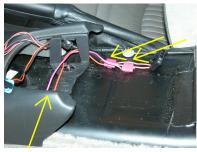
Using one 3M wire tap, connect the pink wire to the pink wire of the fuel door switch cable, and then with a second 3M wiretap, connect the orange wire to the orange wire of the fuel door switch cable.
